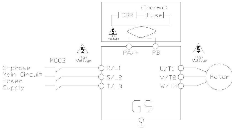
Fig.29. Braking resistor circuit with a thermal fuse
