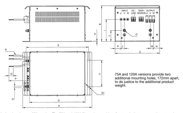
Note: This drawing shows a 25A version. The 75A and 120A filters also provide safety terminals to connect the external supply for the internal cooling fan. These terminals are located next to the connections of the temperature sensor.
