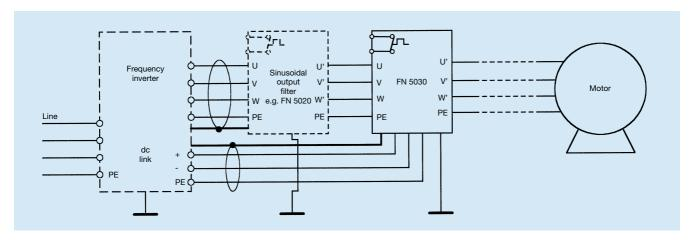
All filters of this range are equipped with a temperature switch. The 75A and 120A versions provide additional internal cooling fan's, which require external supply. Further, this whole series requires the connection to the inverter dc-link in order to develop its full potential.
