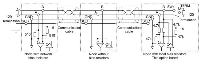
N.B.:Do not connect the SCR terminal to the power ground of inverters or other units. Keep the network cables 20cm or more separate from the power cables to prevent from malfunctioning due to electromagnetic noise.
