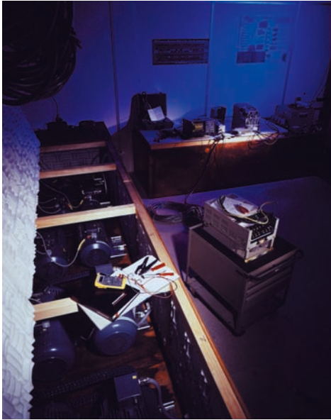
Schaffner's full load test set-up for motor drives
