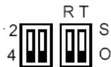
Only the TOSHIBA frequency inverters series VF-S11 at the end of the line must be configured as follows (SW1 and SW2):
